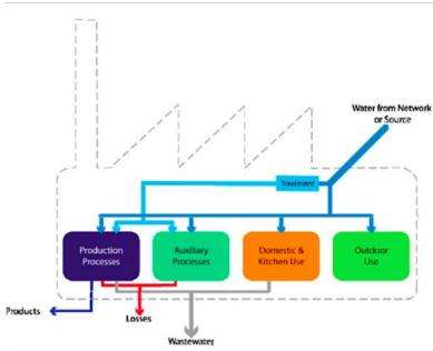
Fig. 4. Water use in industrial plant.
